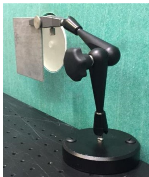
Neutron Transmission Sample in front of Aperture
