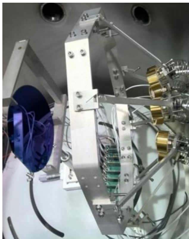
Eight Si detectors mounted inside the NDP vacuum chamber in a ring format
